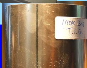
Stainless tube with TIG weld
