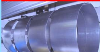
Multiple tube production per machine cycle.
